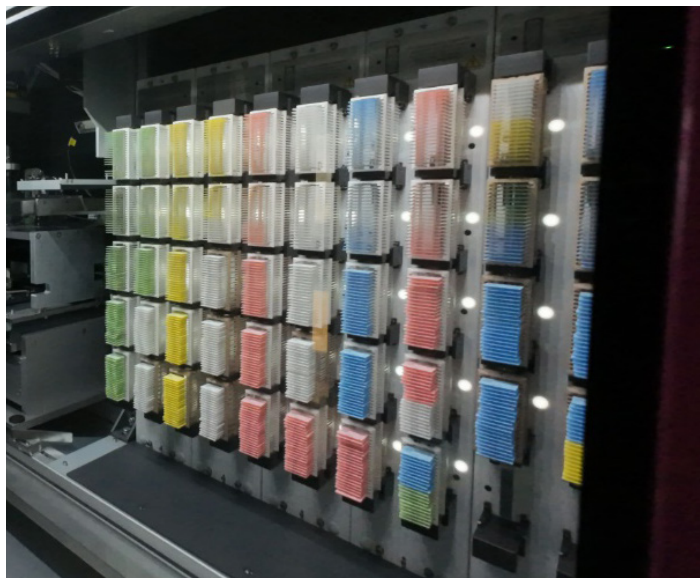
Image 3: Printed slides that have been transferred into slide baskets and loaded into E1000 Dx.
