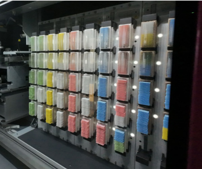
Image 3: Printed slides that have been transferred into slide baskets and loaded into P1000 DX.
